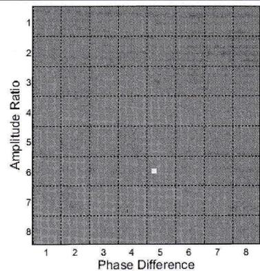
**Figure 7** — All 64 subspaces are combined for displaying in a 128x128 image. The white square indicates a possible location of a signal power in subspace 45. Top-left lowest frequency, bottom-right highest frequency.
