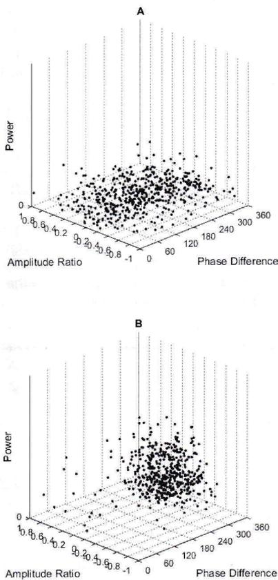
**Figure 5** — The concentration of power in a single bin (23 Hz bandwidth) of only noise (A) on both antennas and the same noise with a circularly polarized signal with 3 dB SNR (B). Each dot is one of 4x125 measurements over 4 seconds.
