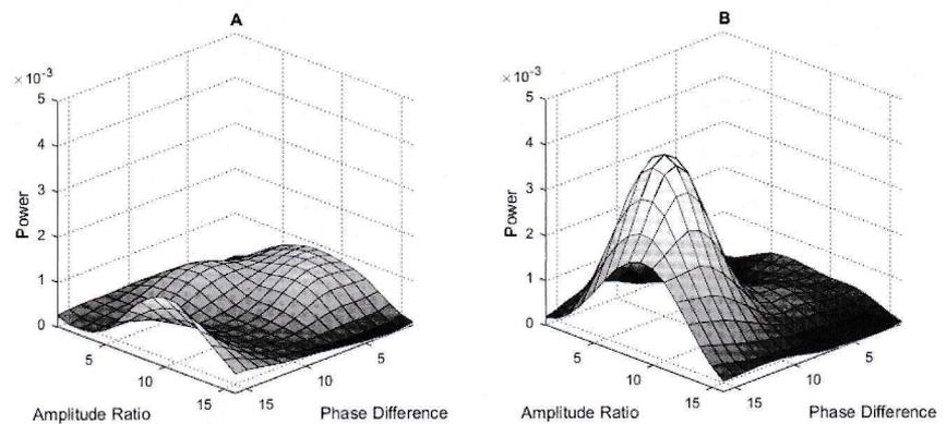
**Figure 11 — The effect of combining a time filter and subspace low-pass filter in a SSB subspace with (A) only noise and, (B) with a circular polarized signal at 3 dB SNR.**
