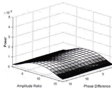
Figure 13 — The scaled sampled noise floor as a result of combining time filtering and space filtering of only noise.
