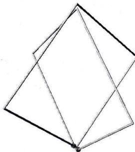
Figure 1 — Two orthogonal small active receiving loop antennas, each 1.25 m by 1.25 m.
