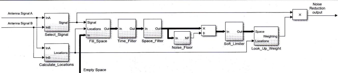
Figure 3 — Noise reduction processing using a 3D space.
