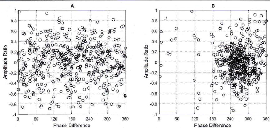
Figure 4 - The concentration in space in a single bin (23 Hz bandwidth) of just noise on both antennas (A), and the same noise with a circular polarized signal with 3 dB SNR (B). Each dot is one of  $4 \times 125$  measurements over 4 seconds.
