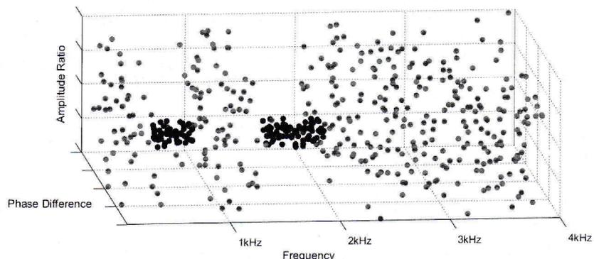
Figure 2 — Possible locations of a SSB signal power with noise over a short period of time in the 3D space.
