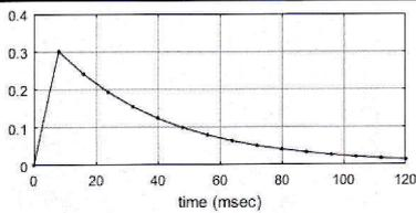
**Figure 8 — The RC-like low-pass time filter default response over 120 ms on a single measurements with amplitude of 1.**
